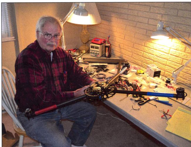
Perritt working on the structure of the Movonator, a 15 lb octocopter that he's building with Sprague as a test platform for specialized mission equipment.
