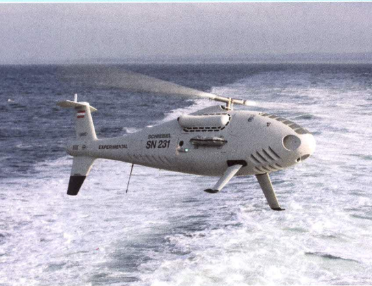
Schiebel's Camcopter has 6 hrs of endurance, a maximum takeoff weight of 440 lbs and can fly as fast as 140 mph.
