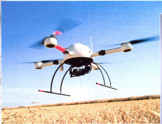
With a flight time of up to 88 minutes, the md4-1000 microdrone was engineered as a geoinformatics tool, to survey and map land areas from the air.
